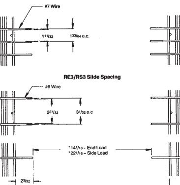
\*181/4 Clearance Between Stop – End Load \*261/4 Clearance Between Stop – Side Load
